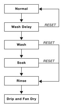
Figure 7 - RESET Mode Sequencing
